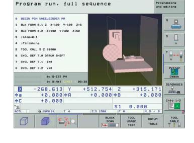
Now the machine manufacturers, too, can develop kinematic tables more quickly. With KinematicsDesign, the user now has a PC tool that gives him graphic support when defining kinematic tables. KinematicsDesign makes it possible to simulate critical axis positions during the conception phase and avoid them by setting limit switches at the right positions on the machine.
